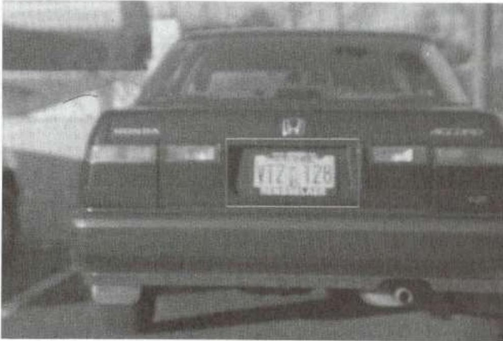
Fig. 8.5. The “license plate” image which is moderately blurred due to an out-of-focus camera, with the area of interest indicated by the frame
